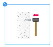
Hammer a screw anchor into each hole.
