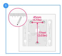
Mark installation hole locations on the wall.
