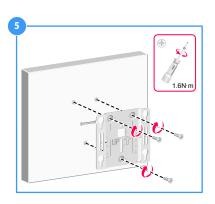
Use screws to attach the mounting bracket to the wall.
