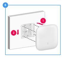
Align the pegs at the device rear with the keyhole slots on the mounting bracket, and rest the device on the bracket. Then, slide down the device until it clicks into place.
