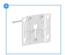
Install the M3  $\times$  23.5 mm security screw to the mounting bracket. Make sure the screw does not block the keyhole slot.
