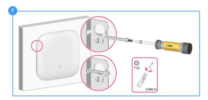
Use the Torx screwdriver to fasten the M3  $\times$  23.5 mm security screw.
