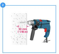
Drill three holes with a diameter of 6 mm (0.24 in) at the marked locations.
